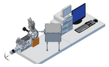
Technical drawing showing full layout of 4 system including light source, camera, control units and PC. Turbo-molecular pump not visible but attaches to base of system
