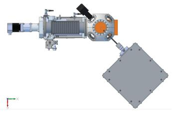
Plan view showing motorized sample stage, spherical chamber and light source at 45°
