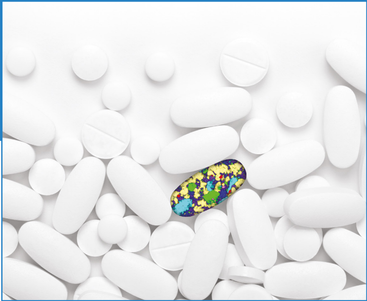
Pharmaceutical tablet compounds distribution based on Raman spectral mapping from low to high concentrations (0.1% to 100%)
