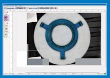
Measurement with CAD (DXF) data overlay
