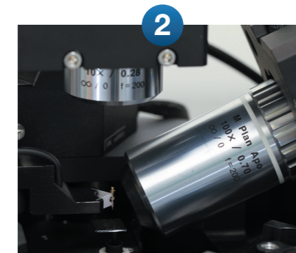
High collection: Wide optical access High numerical aperture objectives for both top and side illumination
