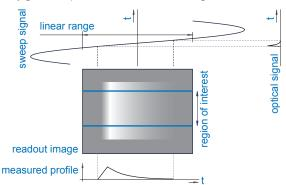
Measurements with positive but also negative time axis are possible. Combined with orthogonal sweep this can be used to capture pulses with double the repetition frequency than sweep frequency.
