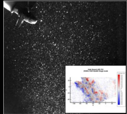
Original and processed data of a PIV measurement showing the flow induced by a ship propeller. Courtesy of ILA\_5150 GmbH.
