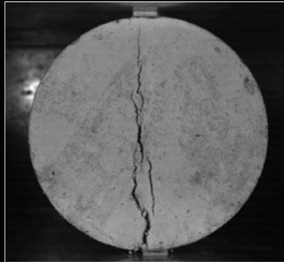
Image of a tensile splitting strength test to characterize the tensile strength of ultra-high performance concrete. Courtesy of TU Braunschweig, iBMB, Division of Concrete Construction.
