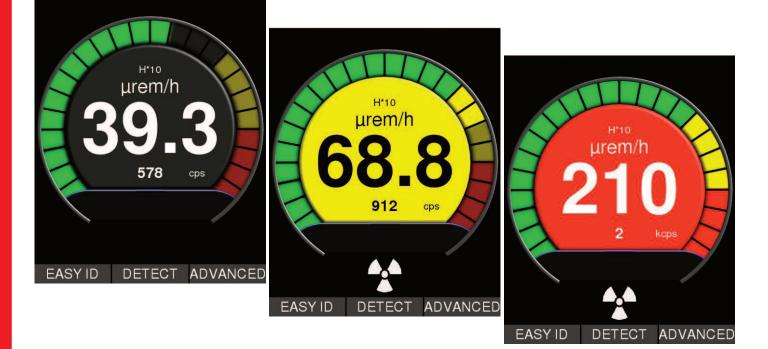
The Detect measuring mode is a tool to locate radiation sources by giving rapid visual and audio feedback to the changing dose rate of incoming radiation. After switching to Detect mode, the user can localize the radiation source by monitoring (in real-time) the auto-scaling chart with color enhanced areas representing the dose rate history of the last few seconds. When the source has been localized, the user may then initiate an "Easy ID" to quickly identify radiating nuclides.
