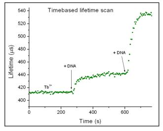
The binding kinetics of Tb3+ to DNA can be followed free of intensity artifacts by using the unique Timebased Lifetime Scan. Here the EasyLife<sup>TM</sup> L performs continuous rapid measurements of the average terbium lifetime in real time.
