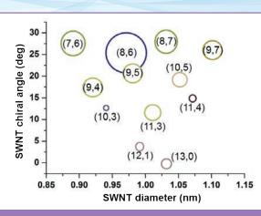
Emission-excitation scan of a mixture of single-walled carbon nanotubes. Plot A is the spectral landscape recorded by the Nanolog; plot B is the structural assignment determined by the Nanosizer software. Diameters and colors of circles in plot B are related to peak-intensities in plot A.
