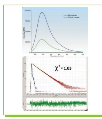
Using the Microsense, 5  $\mu\text{L}$  of AlexaFluor 488 labeled IgG is enough to get steady state or TCSPC data.
