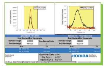
High precision absolute quantum yield characterization of a quantum dot sample enabled by the Quanta- $\phi$  integrating sphere accessory.
