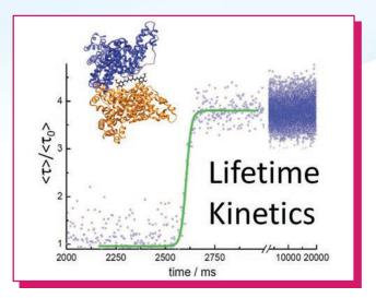
Sample photobleaching corrupts kinetic data by adding an exponential term. Lifetimes are more robust than steady-state intensities. To support rapid kinetics, the Fluorolog-3 is capable of measuring a complete lifetime decay in as little as every 10 ms. Example shown is the binding of Curcumin to Serum Albumin.
