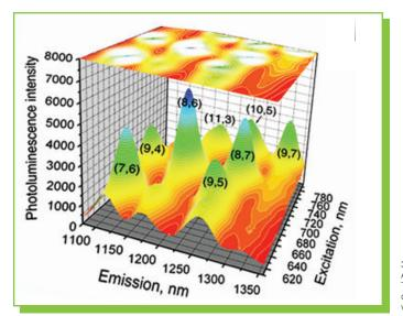
3D EEM of SWCNT acquired with an InGaAs array. Acquisition time for this experiment was <10 minutes. The same experiment can be performed with a single channel InGaAs detector, but the acquisition time would be up to 2 hours for comparable data quality.
