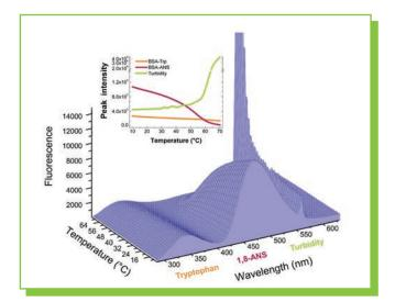
Thermal unfolding of Bovine Serum Albumin in PBS and 1,8-ANS followed using three observables: the quenching of intrinsic Tryptophan fluorescence by water, the quenching of the 1,8-ANS, and the increased 2nd order scattered light which reports turbidity from protein aggregation.
