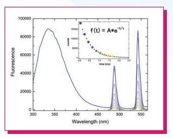
Complex solutions like this mixture of Bovine Serum Albumin (BSA) and Terbium Chloride (Tb<sup>3+</sup>) can be challenging to interpret. Using the pulsed light source of the phosphorescence option allows you to temporally "gate out" the BSA fluorescence, leaving only the Tb<sup>3+</sup> phosphorescence. Inset shows the single wavelength phosphorescence decay of Tb<sup>3+</sup> in this mixture; colored circles correspond to the gated spectra in the main figure.
