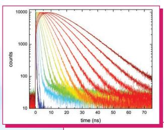
Lifetimes of Rhodamine 6 G in Methanol measured using optional ultrafast PPD detector. At high concentrations, selfquenching results from homodimers and trimers formation. Lifetimes as short as 75 ps are seen, as well as homo-FRET at lower concentrations.
