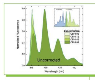
Reabsorption of fluorescence photons can occur even at moderate concentrations, and lead to increasing distortion of spectra with increasing concentration (left). The Fluorolog-3 software can correct this phenomenon, (known as the innerfilter effect), using the sample absorbance measured by the absorbance accessory (right). Add absorbance to your fluorescence measurement.
