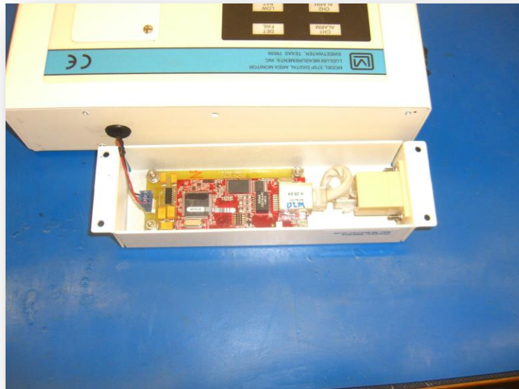
Figure 45 – External Rabbit Ethernet Board Removal
